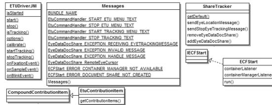
**Figure 1.** Class diagram of the GazeShare architecture
